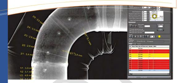
Computed Radiography (CR) is the production of a digital image by using a Phosphor Imaging Plate (IIP) in place of a conventional film.
