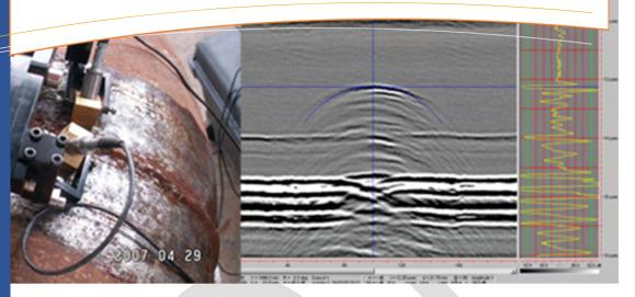
Time of Flight Diffraction or TOFD, is one of the most promising ultrasonic techniques for the examination of welds on pressure vessels in lieu of radiography; for pipe weld quality or crack detection and also weld root erosion. TOFD is a computerized ultrasonic system able to scan, store, and evaluate indications in terms of height (through wall thickness), length and position, with a degree of accuracy and speed never achieved with other ultrasonic techniques.
