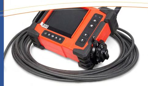
Our Video-probe is equipped with the latest technology in borescopes. A long fiber-optic cable illuminates the inspection area with light generated by a new state-of-the-art lamp in the Light Box. A miniature camera assembly in the viewing tip of the probe then converts the optical image into an electronic image. This image is carried back through the probe cable and displayed in the LCD color monitor. It allows the inspection of surfaces inside narrow tubes or difficult-to-reach chambers.
